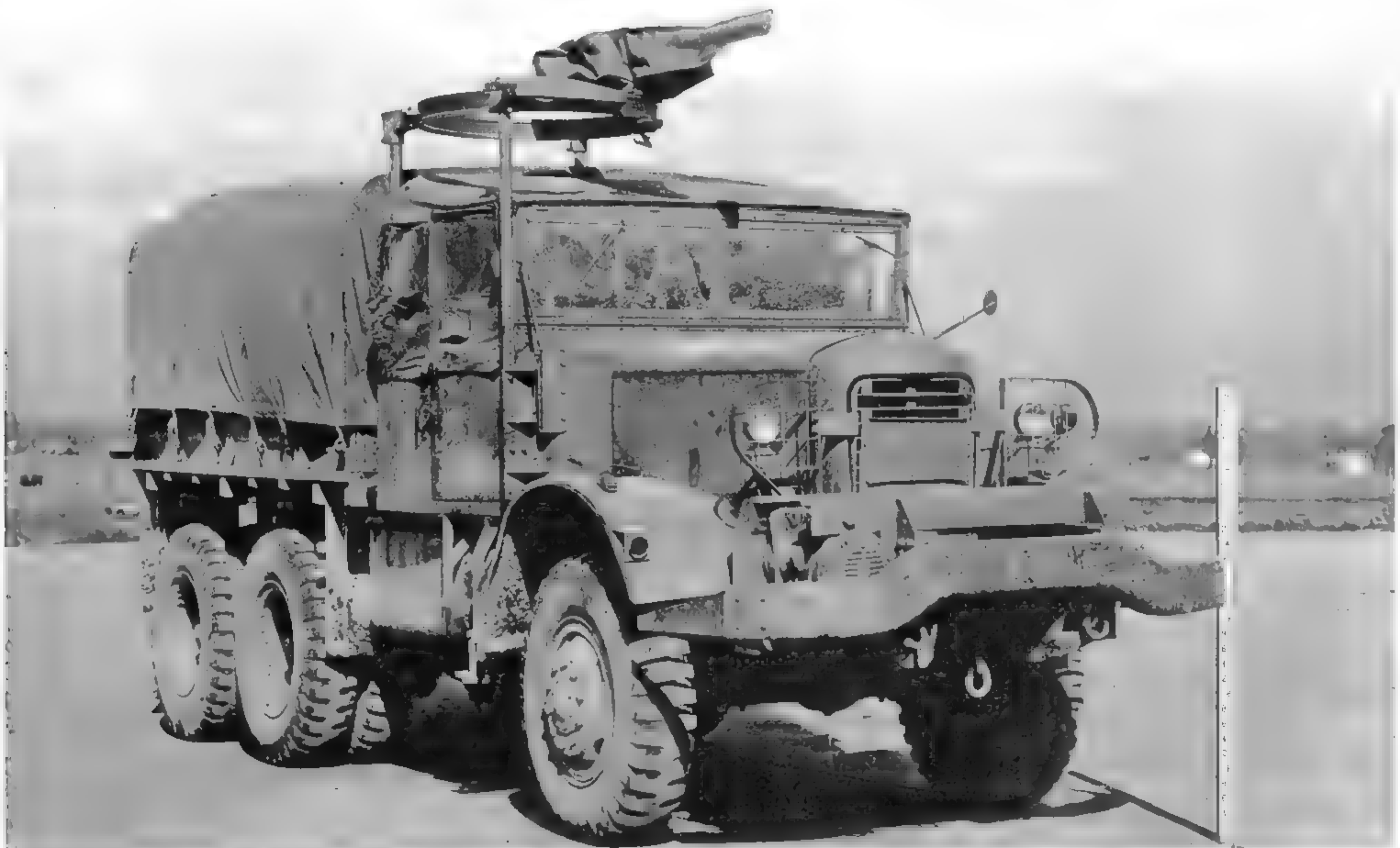
Like most of the open-cabbed tactical vehicles of WWII, the NO could be fitted with the M36 anti-aircraft machine-gun mount. This filthy example was photographed at the Aberdeen Proving Grounds in February 1943. (National Archives and Records Administration photo)
